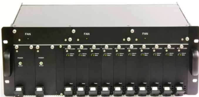
IVE-40; 40 channel rack mountable encoder
