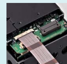
Micro coaxial cable can be used for digital interface.
